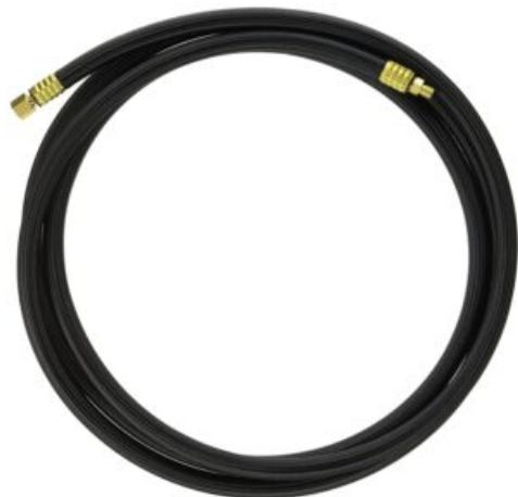
Taurus power cables are manufactured from high-quality copper to the correct torch amperage specification. The Taurus power cable delivers current, shielding gas and welding wire to the front tip of the MIG torch. If the power cable is water cooled, it will also allow water to flow through to the conductor tube for enhanced cooling.
