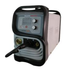
The iWeld MIG-225PA SYNERGIC is a 225A single phase, 220V MIG multi-purpose welding machine which is designed on and manufactured to the latest digital inverter technology. It supports MIG, MAG, LIFT TIG and MMA welding processes. The machine is extremely portable and can accommodate a wire spool of up to 5 kg. It is ideal for on-site work due to its light mass and diverse applications. Its characteristics ideally suit professionals and DIY users.
