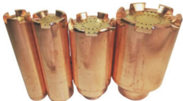
TAURUS 2290-HN heating nozzles are designed for efficient, heavy-duty heating and its flames are ideal for metal-heating prior to welding or bending. The precision engineered and manufactured nozzles are designed to reduce the occurrence of flashbacks. Oxygen and LP/propane gas must be used.
