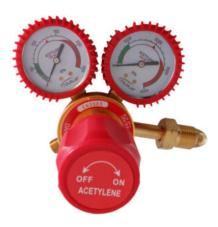
The primary function of a gas regulator is to reduce high-pressure gas in a cylinder or process line to a lower, more usable level. A regulator is not a flow control device. It is used to control delivery pressure only. It has two gauges, one to measure the inlet pressure and the other to measure the outlet delivery pressure.
