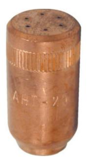
TAURUS AHT-N heating nozzles are designed for efficient, heavy-duty heating and its flames are ideal for metal-heating prior to welding or bending. The precision engineered and manufactured nozzles are designed to reduce the occurrence of flashbacks. Oxygen and Acetylene gas must be used.
