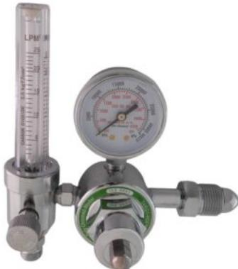
The TARG1-HDFM Taurus heavy duty flowmeter is manufactured from heavy duty brass which connects to an argon gas cylinder. Its function is to measure the amount of gas passing through. It is generally used in TIG and MIG welding. The adjustment knob accurately controls the flowrate but not the pressure.. The flowrate is set in litres per minute. The gauge measures the inlet pressure and the tube measures the delivery flowrate.
