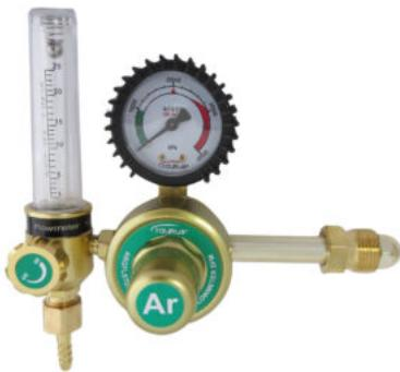
The TAR1SFM and TARG1-CFM Taurus argon flowmeter connects to an argon gas cylinder. Its function is to measure the amount of gas passing through. It is generally used in TIG and MIG welding. The adjustment knob adjusts the flowrate and not the pressure. The flowrate is set in litres per minute. The gauge measures the inlet pressure and the tube measures the delivery flowrate.
