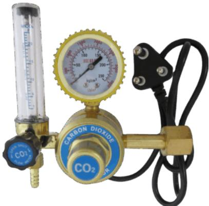
The Taurus CO2 heated flow meter connects to a gas cylinder. Its primary function is to heat the MIG gas mixture containing carbon dioxide and prevent it from freezing. The flowrate is measured in liters per minute and can be adjusted. The inlet pressure is indicated on the gauge.
