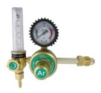
The TAR1SFM and TARG1-CFM Taurus argon flowmeter connects to an argon gas cylinder. Its function is to measure the amount of gas passing through. It is generally used in TIG and MIG welding. The adjustment knob adjusts the flowrate and not the pressure. The flowrate is set in litres per minute. The gauge measures the inlet pressure and the tube measures the delivery flowrate.
