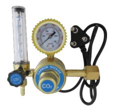
The Taurus CO2 heated flow meter connects to a gas cylinder. Its primary function is to heat the MIG gas mixture containing carbon dioxide and prevent it from freezing. The flowrate is measured in liters per minute and can be adjusted. The inlet pressure is indicated on the gauge.
