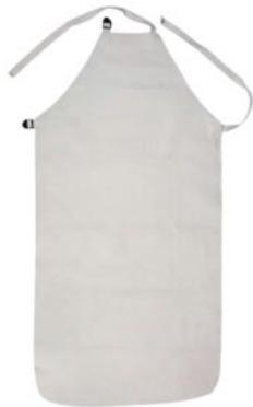
Taurus chrome-coloured leather aprons are one-piece, durable products fabricated from split-grain cowhide leather. It protects clothes and skin against hot metal, slag and fragments generated from welding, grinding and cutting operations.
