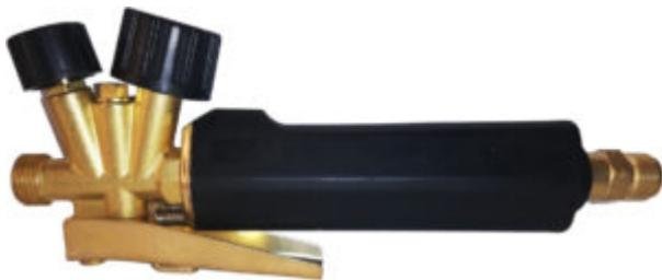
The double-valve handle is designed for a secure hand fit and larger burners are normally fitted. An adjustable economiser valve enables a gas-saving pilot flame. Once the trigger is depressed, the pilot flame instantly shifts to the main flame or to a pulsating main flame. The economiser valve saves both time and gas, especially when working over extended periods with frequent breaks.
