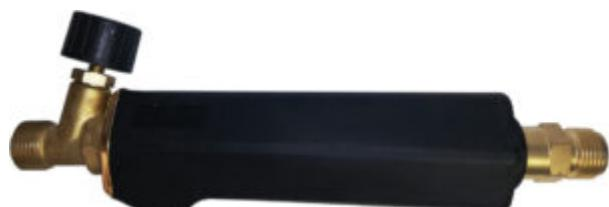
The single-valve torch is designed for a secure hand fit and smaller burners are usually fitted. The main flame will be enabled on ignition since the torch handle is not fitted with a pilot flame device or trigger.
