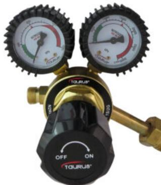
The primary function of a gas regulator is to reduce high-pressure gas in a cylinder or process line to a lower, more usable level. A regulator is not a flow control device. It is used to control delivery pressure only. It has two gauges, one to measure the inlet pressure and the other to measure the outlet delivery pressure.
