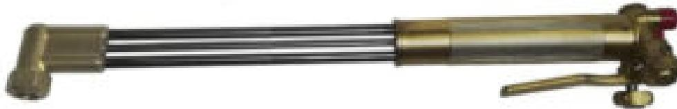
The Taurus MOD28 a 500mm heavy-duty, versatile and robust cutting torch has a 90 degree angled head. Taurus 2890-F or 2890-P threaded nozzles must be fitted. The torch can cut through steel up to 300mm thick. Oxygen and acetylene or oxygen and LPG or propane gas can be used.
