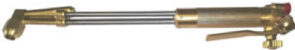
The Taurus 62-3F 500mm long heavy-duty versatile and robust cutting torch has a 90 degree angled head. Flat base Taurus NX nozzles must be fitted. The torch can cut through steel up to 300mm thick. Only oxygen and LPG or propane gas can be used.
