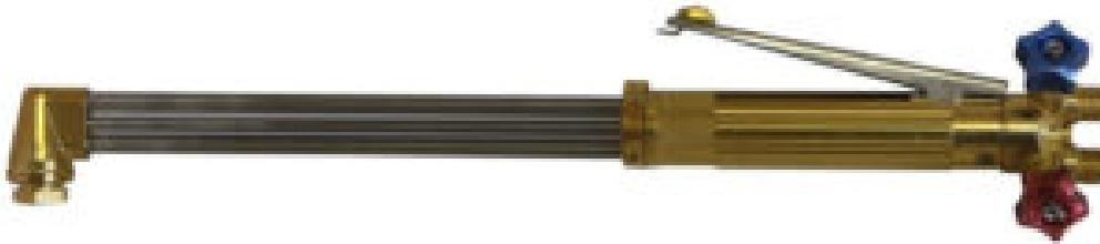
The Taurus universal 500mm long cutting torch is a heavy-duty, versatile and robust Saffire style torch with a 90 degree angled head. It can cut through steel up to 300mm thick and ANM, ANME, PNM or PNME nozzles can be fitted. Preheated oxygen and fuel gas mixed in the nozzle ensure greater safety and higher backfire resistance.
