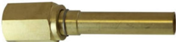
The application of the TYPE 2 UNIVERSAL MIXER is for gas welding/brazing and for heating. It requires to be fitted to the Taurus UNIVERSAL SHANK and uses MK2 swaged brazing nozzles. Oxygen and acetylene or oxygen and LP gases are supported.
