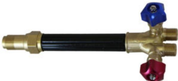
The Taurus Type 2 universal shank can only be used in conjunction with either the TYPE 2 cutting attachment, the TYPE 2 mixer or the TYPE 2 high capacity mixer and the selection depends on the task at hand. It has a steel cutting capacity of up to 150mm thick and oxygen, acetylene and LP gases are supported. The inlet connections are 3/8" BSP.
