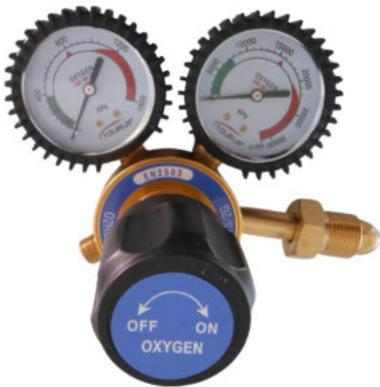
The primary function of a gas regulator is to reduce high-pressure gas in a cylinder or process line to a lower, more usable level. A regulator is not a flow control device. It is used to control delivery pressure only. It has two gauges, one to measure the inlet pressure and the other to measure the outlet delivery pressure.
