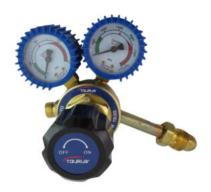
The primary function of a gas regulator is to reduce high-pressure gas in a cylinder or process line to a lower, more usable level. A regulator is not a flow control device. It is used to control delivery pressure only. It has two gauges, one to measure the inlet pressure and the other to measure the outlet delivery pressure.
