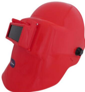
Taurus flip-front welding helmets are manufactured from polypropylene and are suitable for MIG, TIG and arc welding. During the welding operation it protects face and eyes from sparks, light and radiation. Shaded lenses are protected by clear glass lenses. Lenses are 108mm X51mm and are easily replaceable.
