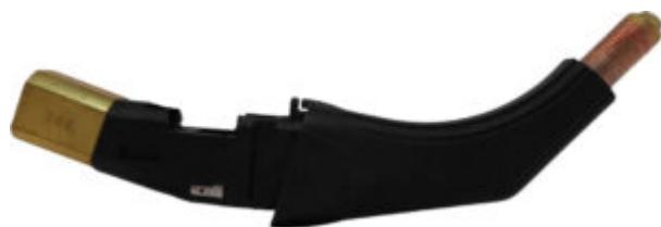
The Taurus XP conductor tube is the extended section protruding from the torch handle on which the head assembly, contact tip and gas nozzle are mounted. The conductor tube delivers the electrical current, filler wire, and shielding gas on to the weld pool.
