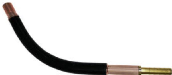
The Taurus TW conductor tube is the extended section protruding from the torch handle on which the contact tip and gas nozzle are mounted. The conductor tube delivers the electrical current, filler wire, and shielding gas on to the weld pool. Conductor tubes are also known as swan necks or goose necks.
